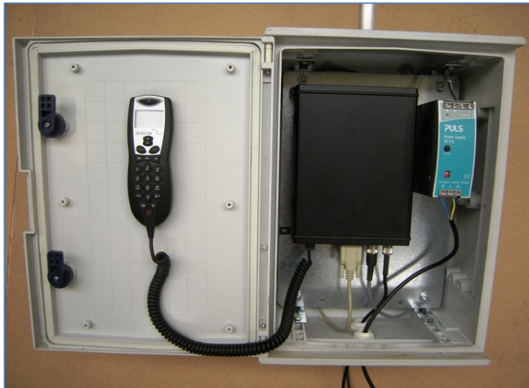
Typical enclosure suitable for deploying MiChroSat 2403 in an Outdoor Environment
